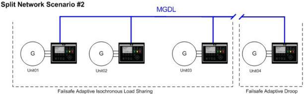
Scenario 1. If a controller (Unit 01, for example) detects fewer than half the expected number of controls online (a minority), then the minority operate in the Failsafe Adaptive Droop mode and the balance in the Failsafe Adaptive Isochronous Load Sharing mode.
