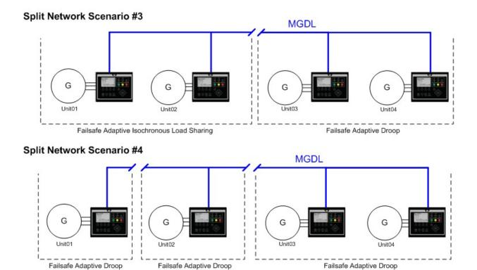
Scenario 3. If a controller detects exactly half the expected number of controls on the network, there are two possibilities. If the control detects the lowest unit number, then that unit and the other units in its half operate in Failsafe Adaptive Isochronous Load Sharing mode, and the other half operate in the Failsafe Adaptive Droop mode. If the control does not detect the lowest unit number, the opposite occurs.
